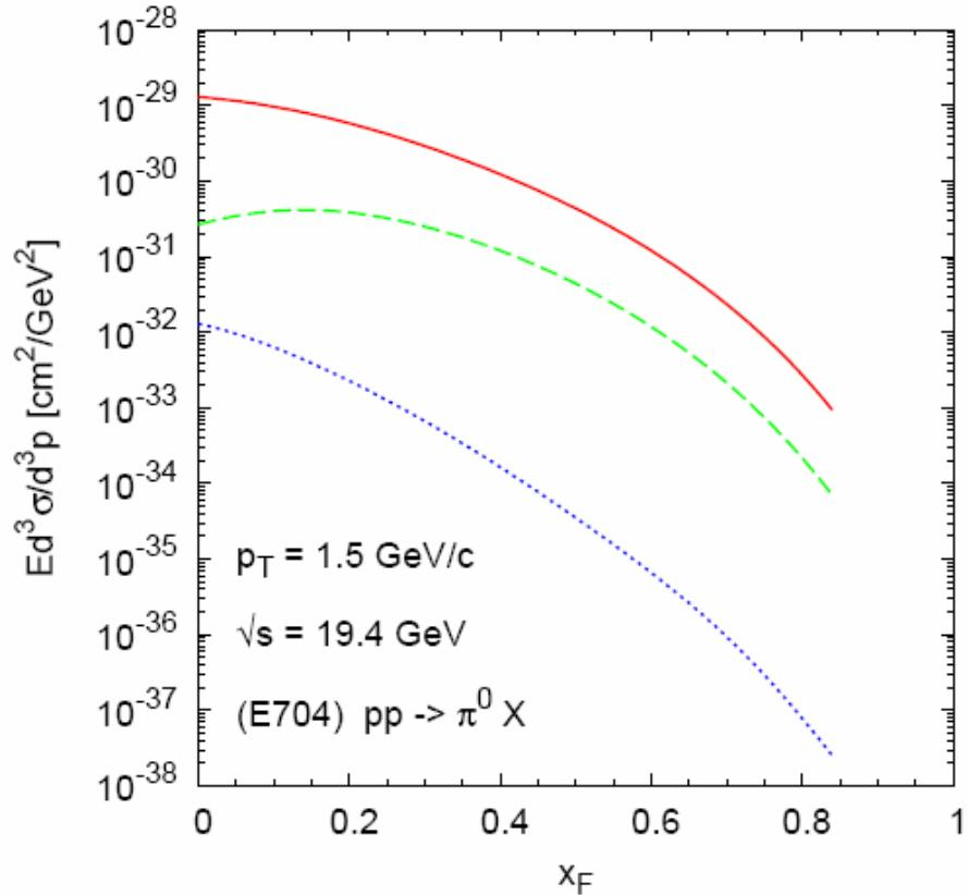
Contributions to the unpolarized cross section, plotted as a function of  $x_F$  for  $pp \rightarrow \pi^0 + X$  processes and E704 kinematics, as indicated in the plot. The three curves correspond to: solid line = usual unpolarized contribution; dashed line = Boer-Mulders  $\otimes$  Collins contribution (maximized); dotted line = Boer-Mulders  $\otimes$  Boer-Mulders contribution (maximized).
