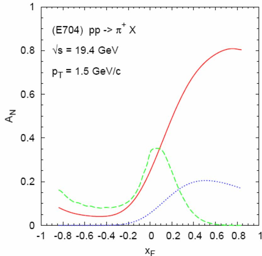
Maximized contributions to the SSA  $A_N$ , plotted as a function of  $x_F$ , for  $pp \rightarrow \pi^0 + X$  processes and E704 kinematics, as indicated in the plot. The three curves correspond to: **solid line = quark Sivers mechanism**; **dashed line = gluon Sivers mechanism**; **dotted line = transversity  $\otimes$  Collins contribution**; all other contributions are much smaller.
